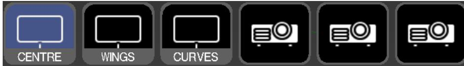
The fixture group is a list of all of the fixtures that have been added to the current show. On the Stage Construction page it will display all fixtures in the system.
