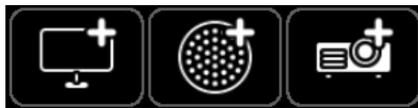
To add a fixture, you simply need to click on the top left menu which has a button for each of the three fixture types along with a plus icon.
