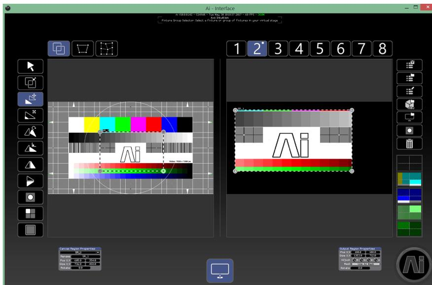
The screen fixture provides an underlying toolset to allow you to create regions, specifying an area on the output to draw to, and what part of the texture to extract from. Where the main unit of control here will be pixels. If a region has inequality
