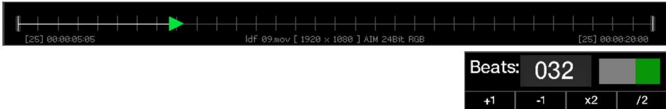
The playback bar allows for you to affect the in/out points of the media as well as allowing you to scrub the current playhead to a given point in time for the media selected. To change the in/out points you simply click on the first or last bar and drag it to the desired location. Clicking anywhere in between and dragging will scrub the playhead position of the media to that point in time.
