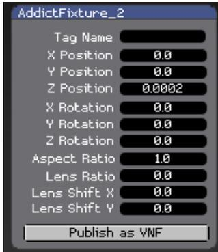
The projector fixture should be used when you intend to do video mapping or vertex editing using a 3D model. It works in conjunction with the Screen Fixture models, by capturing their geometry and then applying adjustments on those based on it's positioning in the Virtual Scene.
