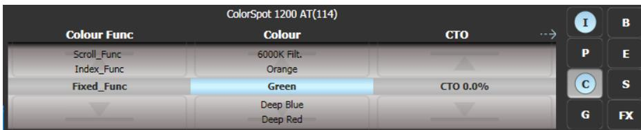
To the right of (Sapphire Touch) or above (other consoles) the roller, the screen shows which attribute group (IPCGBESFX or Intensity, Position, Colour, Gobo, Beam, Effect, Special, FX) is selected (grey box) and which are currently modified (blue circle).
