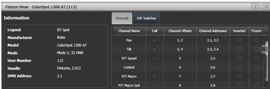
If the fixture address is set using DIP switches, the console can show you how to set the switches by clicking on the DIP Switches tab.
