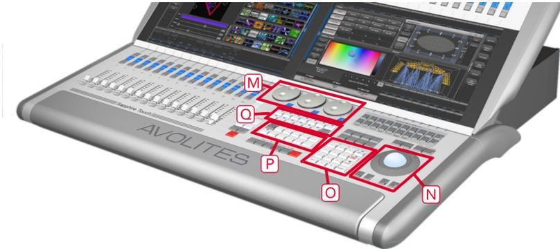
(M) The **Control wheels** are used to set control values (attributes) for the fixtures, and to set chase speeds and fades. The touch screen above the wheels shows information about the attributes being controlled.
