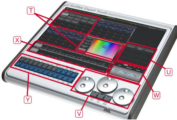
The optional Pearl Expert Touch Wing uses a touch screen and additional wheels to provide the standard Titan interface for selecting fixtures, palettes, groups and setting attributes. It can only be used with the Pearl Expert and connects to the DVI port and the 9-pin D connector on the rear of the console, just above the panel with the rear USB/network sockets.
