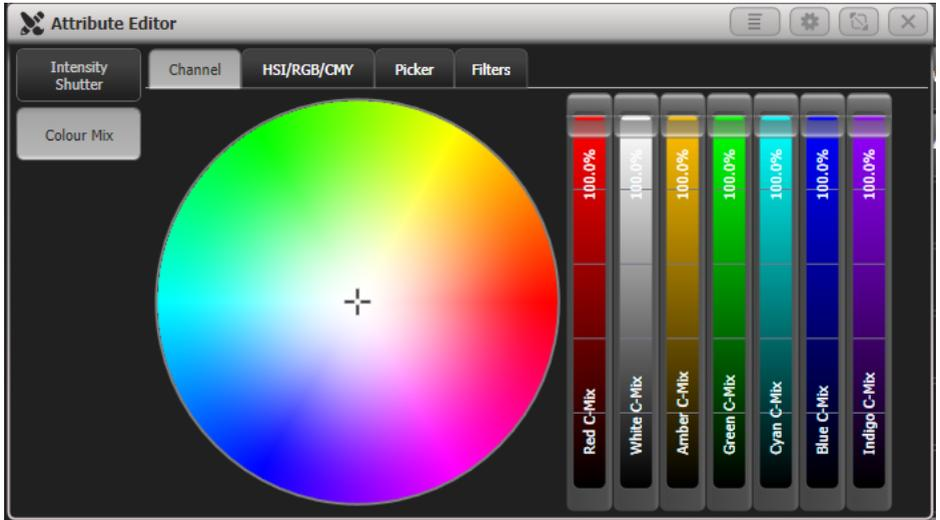
The **Channel** tab provides a colour picker, with a slider for each colour control channel in the fixture. The sliders shown will vary depending on what is provided in the fixture - this example is an ETC Lustr fixture which has 7 independent LED emitter colours. This mode is useful to obtain colours such as tints of white or UV/Congo Blue which are hard to mix from a picker or colour wheel.
