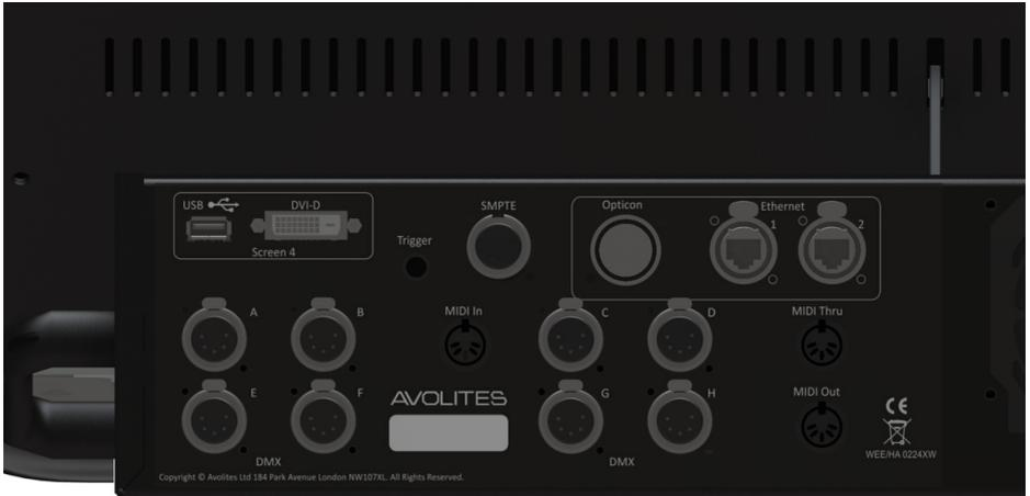
All the connections required for the console are found on the back panel.
