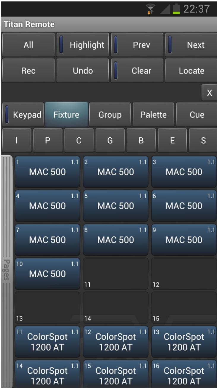
You can connect multiple remotes to the console and the console itself remains functional while the remote is connected. Each remote has a **separate programmer** so an operator can continue to work on the console while another user programs or updates palettes on the remote.
