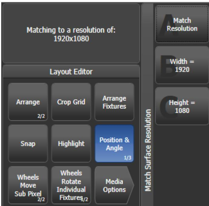
You can also scale fixtures in the Layout Editor to reflect real life size, as the default cell layout from the fixture's personality might not match other fixtures. Toggle the [Position and Angle] context menu button until it shows [Fixture Scale]. If a multi-celled fixture is scaled down to minimum size, the cells will disappear and it will act as a single cell.
