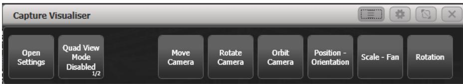
Camera controls are in the Capture Visualiser Settings window (Section 13.2) which you can open by double pressing <Open/View> to show the workspace window buttons, or using the {Open Settings} context button.
