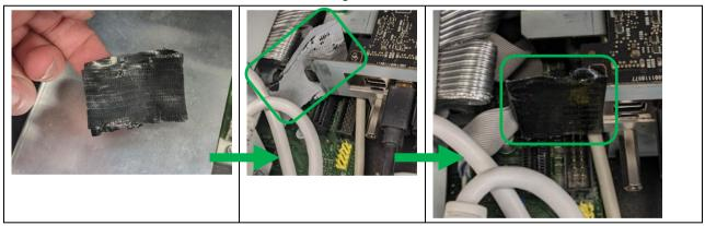
Use two layers of gaffer tape approximately 50x20mm (2 x .78"). Fit behind the PCI Connector as shown, then fold against the frame.
