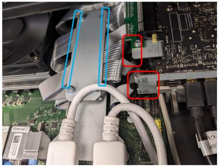
Check that the cables are not touching the frame parts (Red rectangles above) or have been damaged where they touch the retainer (blue rectangle above).
