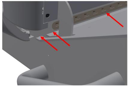
Refit the shell screws and tighten to 0.8Nm.
