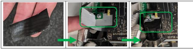
Create two layers strips of gaffer tape approximately 110x20mm (4.3 x 0.78"). Fit between the PCIe cable retainer and the PCIe cable, then fold over the PCI cable retainer, repeat this on the other side.
